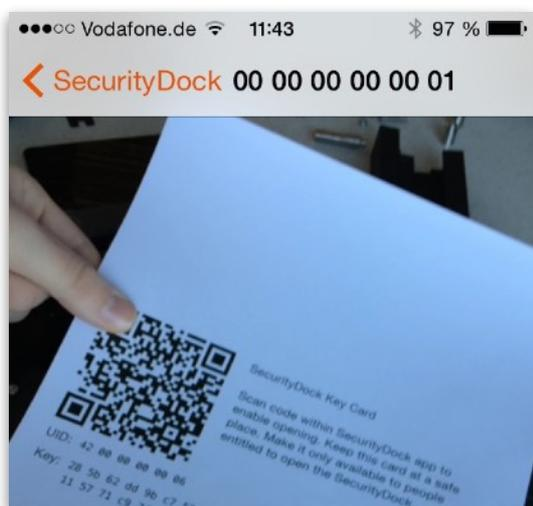
4 Tap the image of your Dock. Your camera is now activated, please allow access for using your camera. To pair your iOS device and your viverooDock, scan the QR code on the included key card. This procedure is necessary only once, after the first pairing the devices are able to communicate with each other. A message indicates the successful pairing of the devices.
