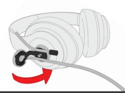
**4.** Using the Tetrakey screw clockwise to secure the Pendant.
