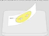
For the adhesive option remove adhesive film and attach to surface.
