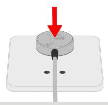
**3**. Insert M5 Screws (not provided) and screw clockwise to secure puck to surface.
