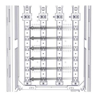
Run the cable up through the hole at the end Pull the cable through the rubber grip. Slide the cable along adjacent to the device
