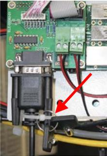
Locate the 3V Lithium battery on the control board, and remove the clear plastic shipping tab. Close and lock the master door.
