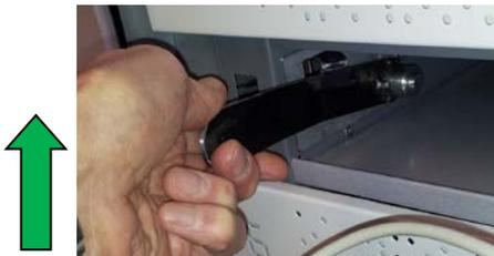
Firmly press up on the lever to release all the doors.
