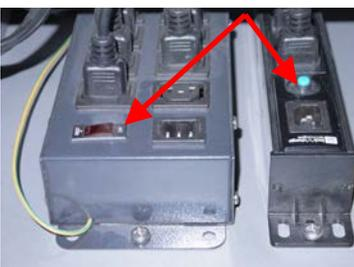
Switch on power to the locker. The controller will take approximately 30 seconds to initialise and boot, and then all fifteen locker doors will be opened sequentially.
