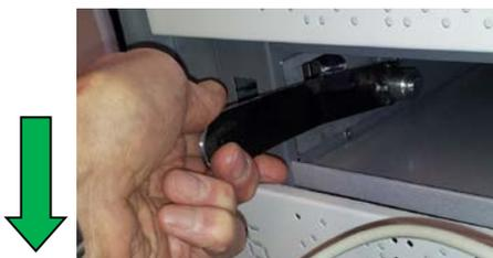
Firmly press down on the lever to reset the release latch.
