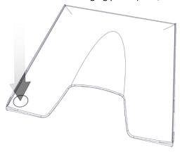
2. The shelf can be removed by lifting gently in the centre and pulling outwards
