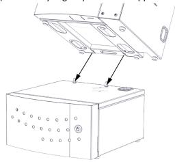
3. Connect the aligning pins to the first Putnam 16 (if applicbable)
