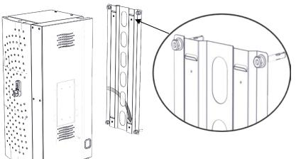
8. Insert 4 securing screws and replace the plastic shelves
