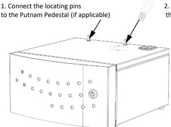
2. Place the first Putnam 16 on the Pedestal aligning to the pins. (or manually align if pins are not applicable)
