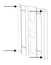
2. Drill holes in the marked in the marked areas. Use a A 10mm masonry drill
