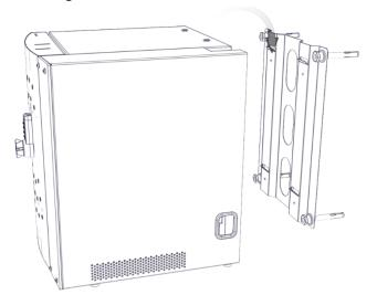
8. Insert 4 securing screws and replace the plastic shelves
