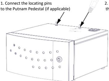
2. Place the first Putnam 8 on the Pedestal aligning to the pins. (or manually align if pins are not applicable)
