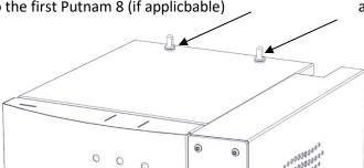
4. Place the second Putnam 8 on the first Putnam 8 aligning to the pins. (or manually align if pins are not applicable)
