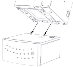
3. Connect the aligning pins to the first Putnam 8 (if applicbable)
