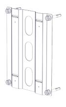
5. Install washers and shear nuts & tighten until the nut shears off
