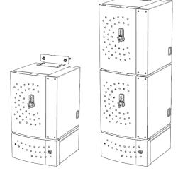
5. Complete the Putnam Stack (Pedestal and two Putnam 8 Charging Stations) by attaching the wall bracket to the Putnam Stack.
