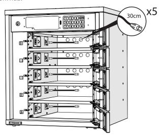
Plug the 30cm ethernet cables to the RJ45 port inside each shelf. Network kit setup for the FUYL Tower 5 is complete.
