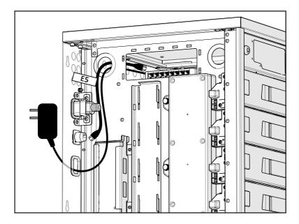
i. Route the hub's power cable through the rear hole to a power outlet. ii. Connect the network hub to the rear internal RJ45 port using the "E5" ethernet cable.
