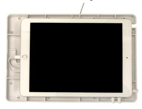
Step 6 – Gently place the front enclosure Make sure the buttons work correctly and the front plate is nicely aligned with the back part of the enclosure.
