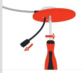
Connect the Standard, Boost or Boost plus power cable to Splitter Puck connection.
