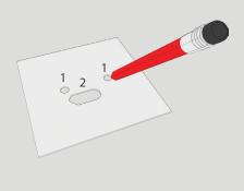
When using adhesive only drill power cable slot (2)
