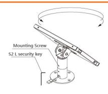
■ Loose the mounting screw with the S2 L security key, then rotate the top tube part to the suitable angle then tighten it with the screw.
