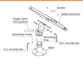
S4 L security key can adjust the tightness of tablet enclosure rotation.
