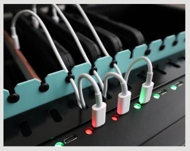
Intelligent charging hub with autom. shut down (no Timer needed) -> works as overheating and overchar ging protection
