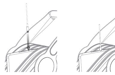
Connect the power cable. Plug cable into cart and into the wall socket\*. The devices will start to charge when power is "On"
